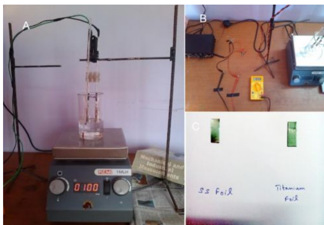
Figure 2. (A) Electrochemical anodizing method Equipments setup in the Lab. (B) DC regulator (C) Titanium foil and Stainless steel foil.
